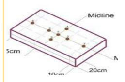
Repeat the hand compression along seven sites as shown in the diagram. Note any variation in the density of the foam, including whether:
