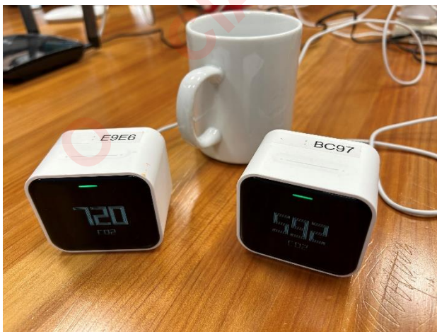
Figure 2-1: Two Qingping Air Monitor Lites of the type used to monitor CO 2 in this study.
